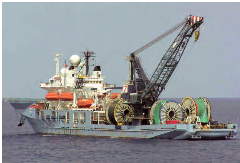
FIGURE 30. Laying of subsea cables
